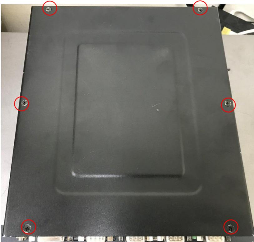
2. Use the 6 M4 screws shipped with the controller to fix the 2 wall-mount brackets, also included, to the chassis, according to the spacing dimensions of the screw holes and brackets, as shown.
