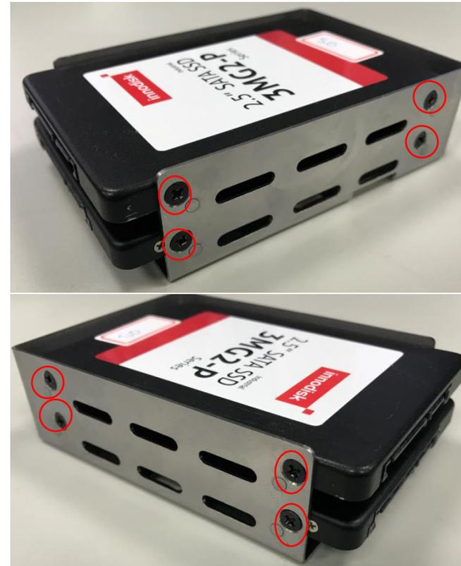
Note: 2.5" HDD or SSD maximum thickness support to 9.5mm
