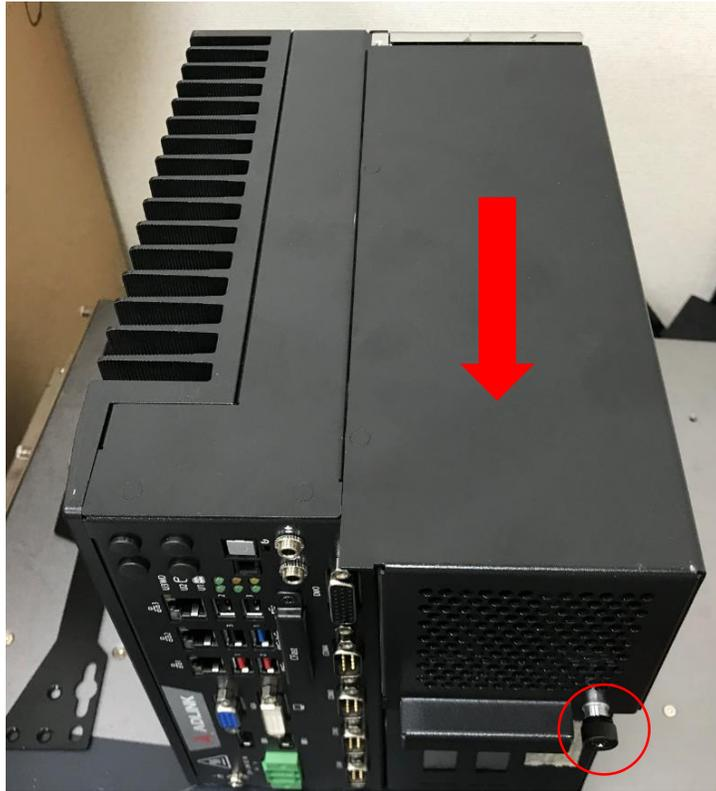
2. Remove the 4 rear base case screws by screwdriver
