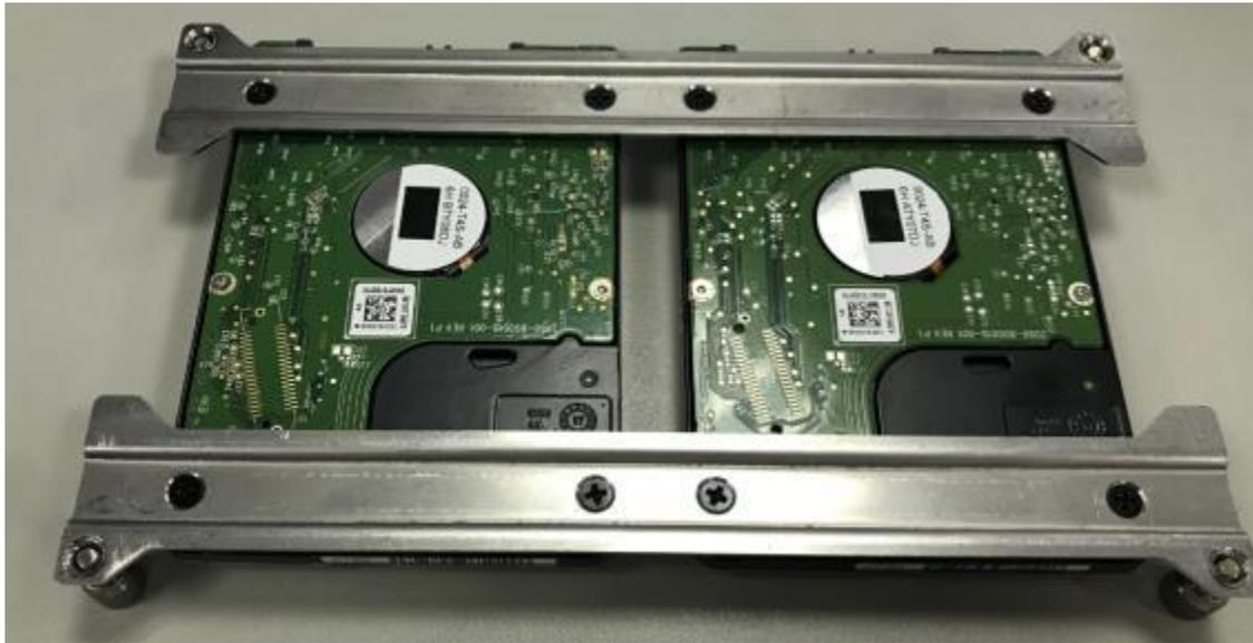
6. Gently seat the drive into the SATA connector on the PCB and 4 hand screws are fix to the bracket.
