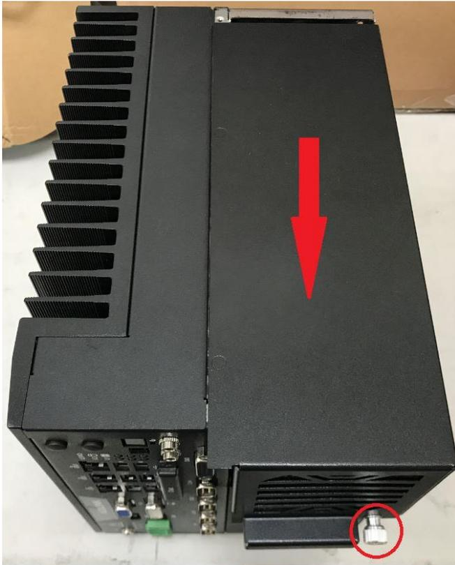
2. Remove the 4 side base case screws by screwdriver.
