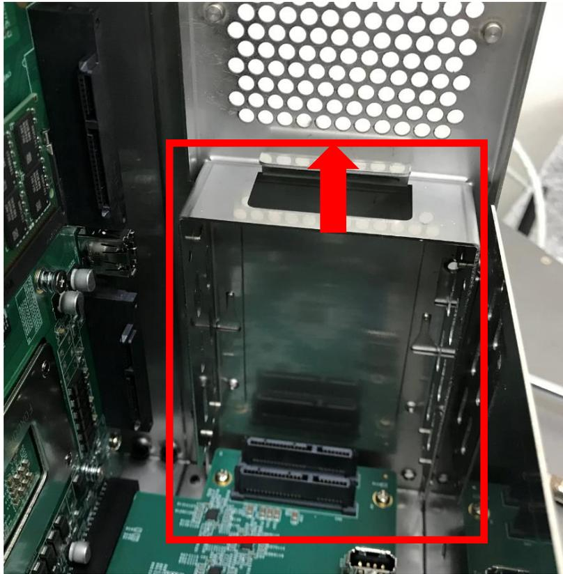
4. Use 8 of the included M3 screws to fix two 2.5" HDD or SSD unit to the bracket.
