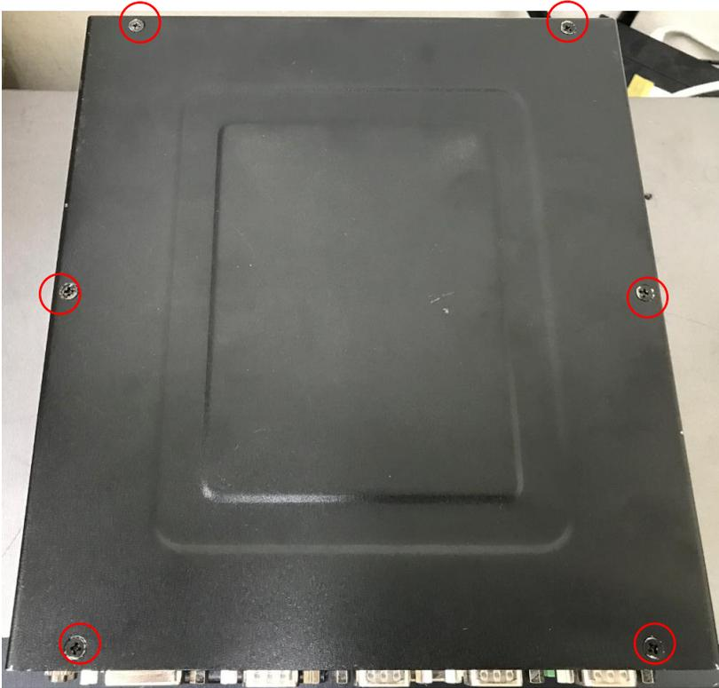
2. Remove the bottom cover by lifting
