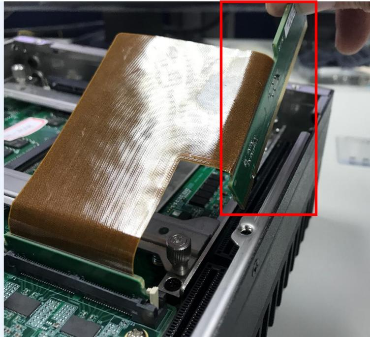
4. Release the hand screw to take the two bracket out.
