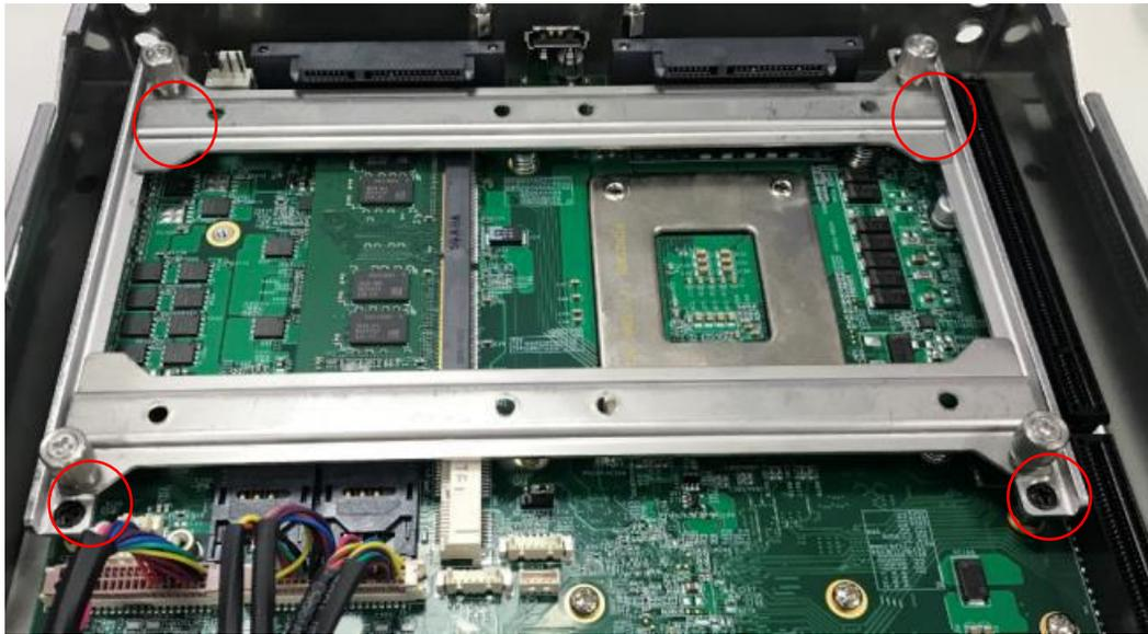
4. Use 8 of the included M3 screws to fix two 2.5" HDD or SSD unit to the Tray from the accessory pack.
