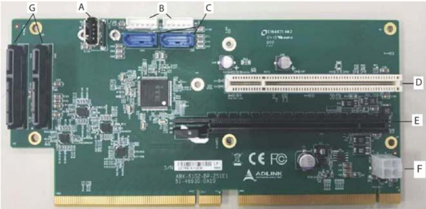
Figure 3-13: 2-slot Backplane Card
