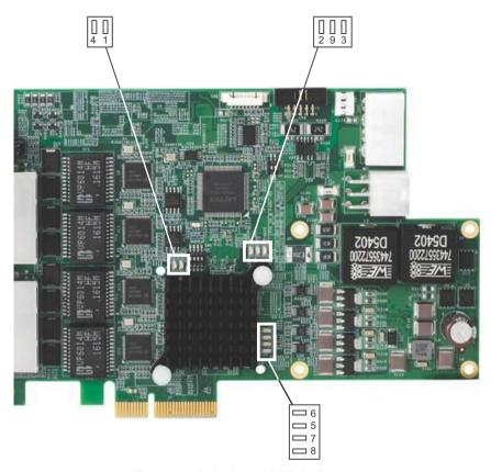
Figure 1-15: Onboard LED Indicators
