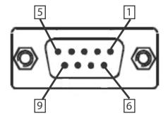
Figure 1-17: I/O Bracket Trigger Connector
