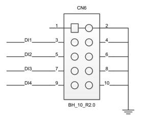
Figure 1-16: Onboard Trigger-in Connector
