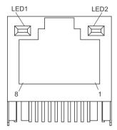
Figure 1-9: RJ-45 Ethernet Connector
