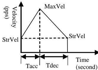
This kind of speed profile could be applied on velocity mode, position mode in one axis or multi-axes linear interpolation and two axes circular interpolation modes.
