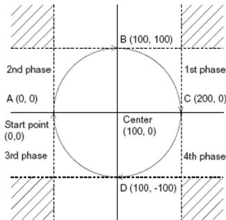
The command precision of circular interpolation is shown below. The precision range is at radius  $\pm 1/2$  pulse.
