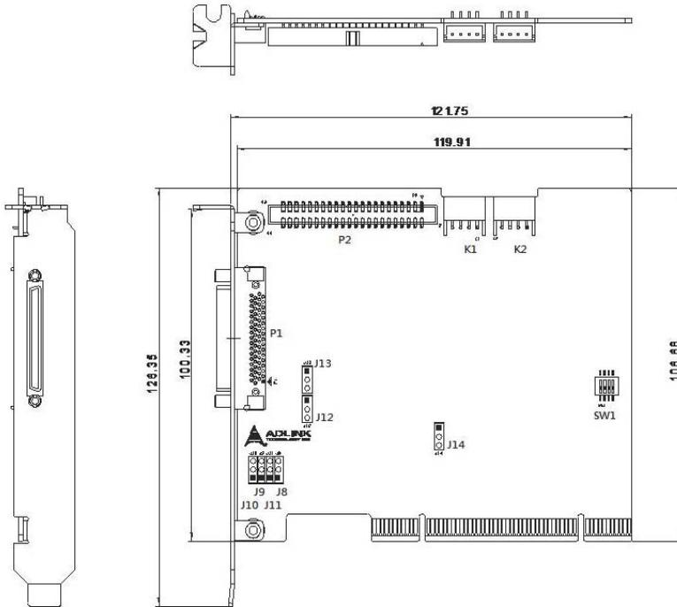
**Figure 2-1: PCB Layout of the PCI-8102**
