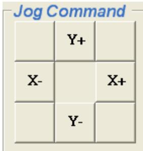
Continuous Jog means that when you press one directional button, the axis will continuously move with an increasing speed. The longer you press, the faster it runs. When you unpress the button, the axis will stop immediately.
