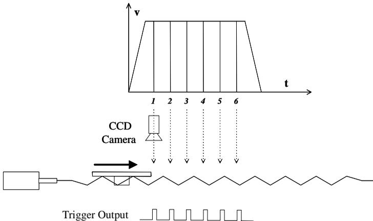
In this application, the table is controlled by the motion command, and the CCD Camera is controlled by CMP pin. When the comparing position is reached, the pulse will be outputted and the image is captured. This is an on-the-fly image capture. If users want to get more images during the motion path, try to set a new compar-
