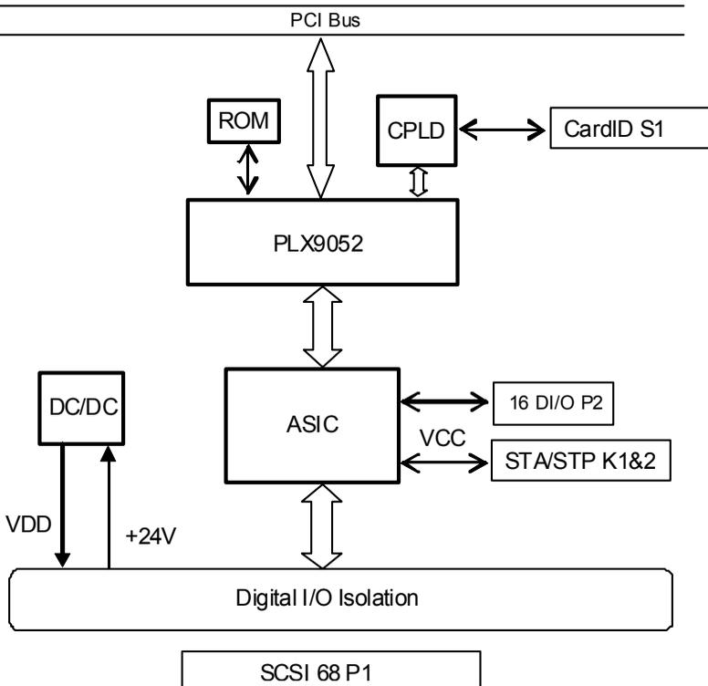
**Figure 1-1: PCI-8102 Block Diagram**
