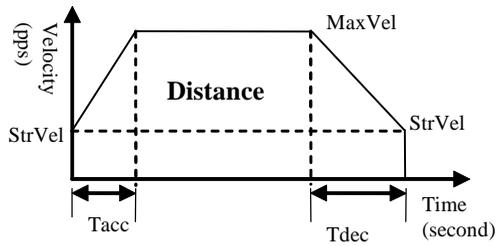
The distance is the area of the V-t diagram of this profile.
