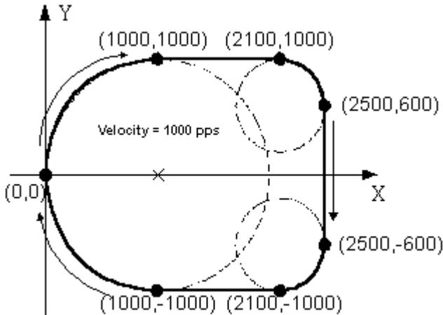
If the INP checking is enabled, the motion will have some delayed between each command in buffers. INP check enabled make the desired point be reached but reduce the smoothing between each command. If users don't need this delay and need the smoothing, please turn INP checking off.
