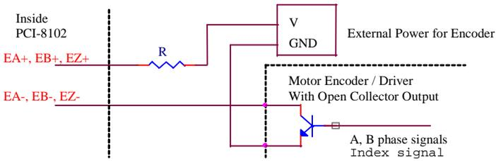
For more operation information on the encoder feedback signals, refer to section 4.4.
