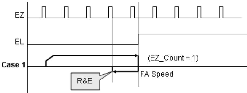
**Home mode=8: (EL On then reverse to count EZ number and reset counter, not using FA Speed)**
