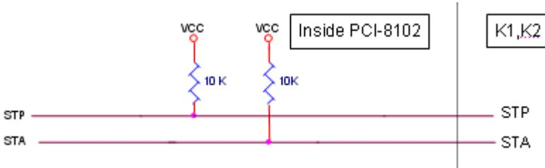
The STP and STA signals are both input and output signals. To operate the start and stop action simultaneously, both software control and external control are needed. With software control, the signals can be generated from any one of the PCI-8102. Users can also use an external open collector or switch to drive the STA/STP signals for simultaneous start/stop.
