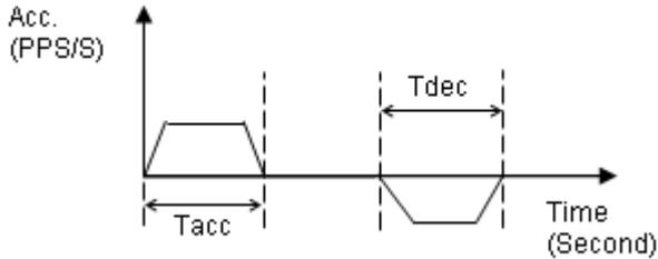
The S-curve profile motion functions are designed to always produce smooth motion. If the time for acceleration parameters combined with the final position don't allow an axis to reach the maximum velocity (i.e. the moving distance is too small to reach MaxVel), then the maximum velocity is automatically lowered (see the following Figure).
