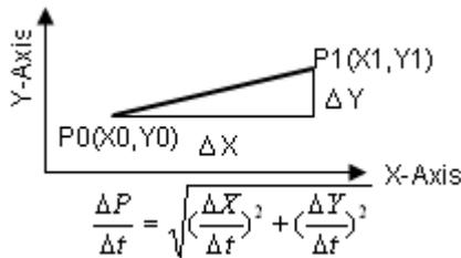
When calling 2-axis linear interpolation functions, the vector speed needs to define the start velocity, StrVel, and maximum velocity, MaxVel.
