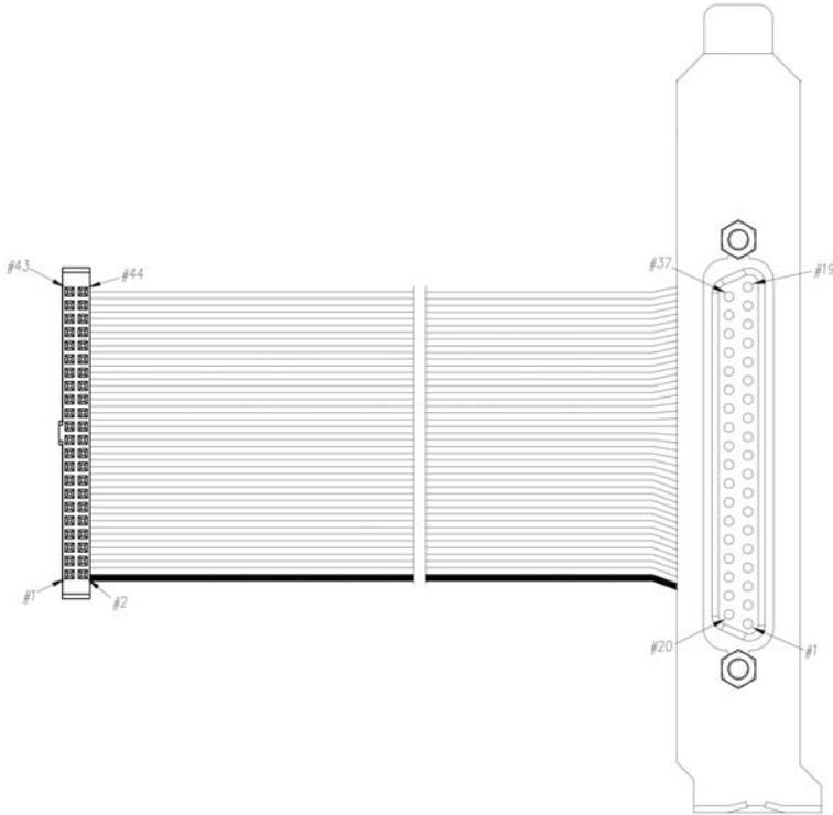
Pin assignment of the DSUB-37p connector is as follows.
