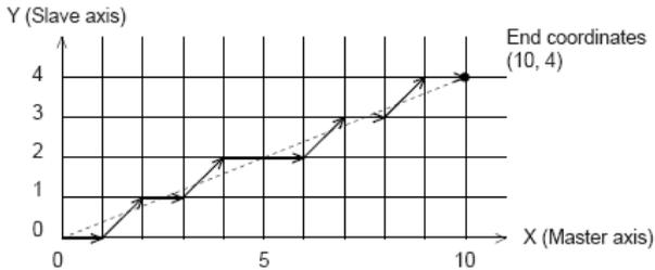
The pulses output from X or Y axis remains 1/2 pulse difference according to a perfect linear line. The precision of linear interpolation is shown as below:
