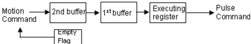
Besides position command, the speed command should be set correctly to perform a speed continuous profile. For the following example, there are three motion command of this continuous
