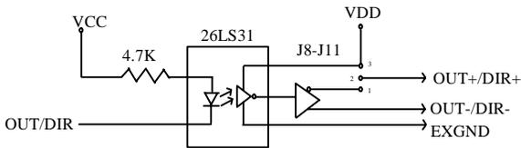
**NOTE:** If the pulse output is set to open collector output mode, OUT- and DIR- are used to transmit OUT signals. The sink current must not exceed 20mA on the OUT- and DIR- pins. The default setting of jumper is 1-2 shorted. The default setting is 1-2 shorted.
