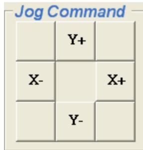
**Incremental Jog:** Incremental jog means that when you click one directional button, the axis will step a distance according to the Step-Size's setting.
