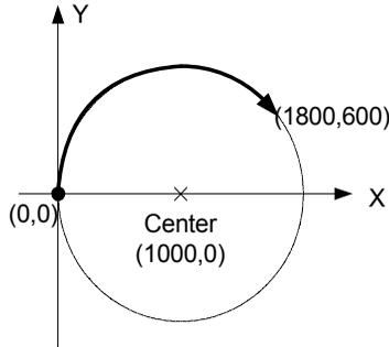
The motion controller will move to the final point user desired even this point is not on the path of arc. But if the final point is not at the location of the shadow area of the following graph, it will run circularly without stopping.
