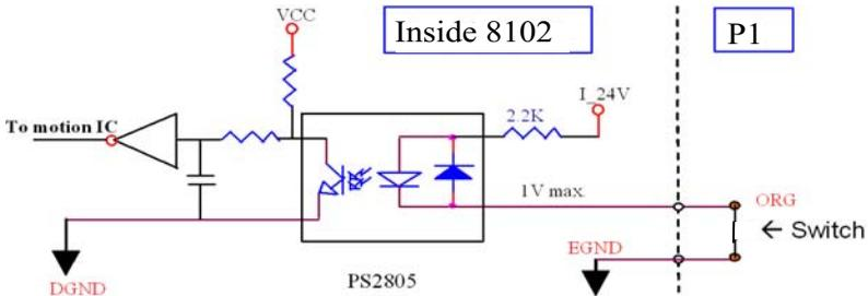
When the motion controller is operated in the home return mode, the ORG signal is used to inhibit the control output signals (OUT and DIR). For detailed operations of the ORG signal, refer to section 4.3.
