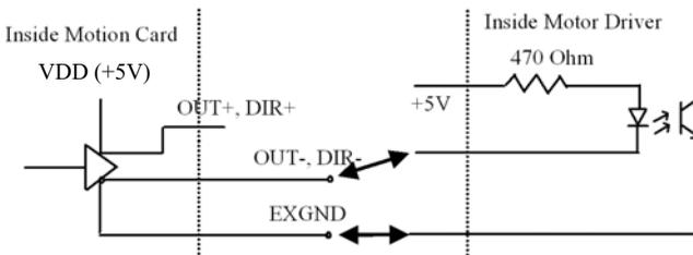
**Warning:** The sink current must not exceed 20mA or the 26LS31 will be damaged.
