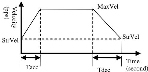
The area of the velocity profile represents the distance of this motion. Sometimes, the profile looks like a triangle because the desired distance from user is smaller than the area of given speed parameters. When this situation happens, the motion controller will lower the maximum velocity but keep the acceleration rate to meet user's distance requirement. The chart of this situation is shown as below:
