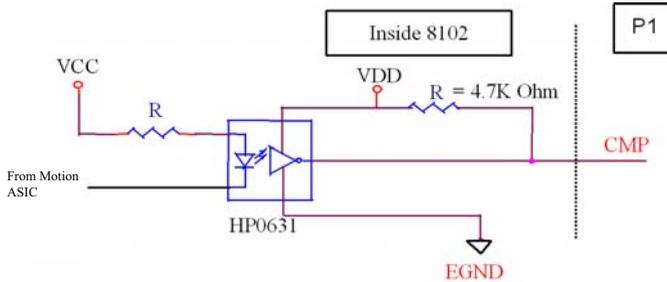
Note: CMP trigger type can be set as normal low (rising edge) or normal high (falling edge). Default setting is normal high.
