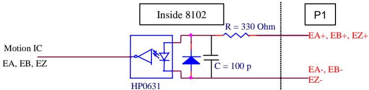
Please note that the voltage across each differential pair of encoder input signals (EA+, EA-), (EB+, EB-), and (EZ+, EZ-) should be at least 3.5V. Therefore, the output current must be observed when connecting to the encoder feedback or motor driver feedback as not to over drive the source. The differential signal pairs are converted to digital signals EA, EB, and EZ; then feed to the motion control ASIC.
