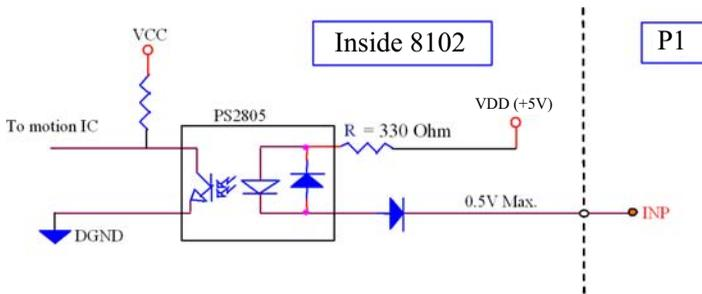
The in-position signal is usually generated by the servomotor driver and is ordinarily an open collector output signal. An external circuit must provide at least 8mA current sink capabilities to drive the INP signal.
