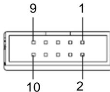
**Figure 2-6: Wafer Connector**
