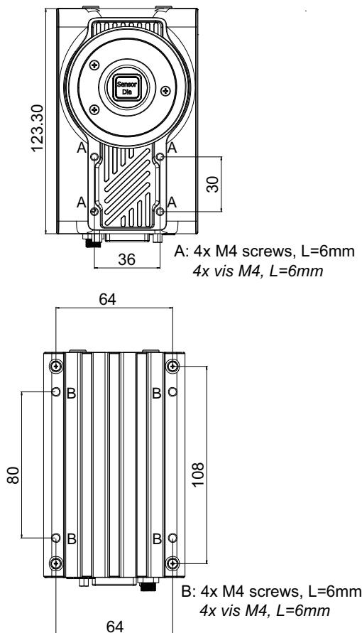
Figure 3-1: NEON-2000-JNX Mounting Holes
