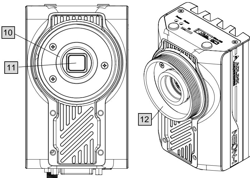
**Figure 2-7: Front Side I/O and Connectors**
